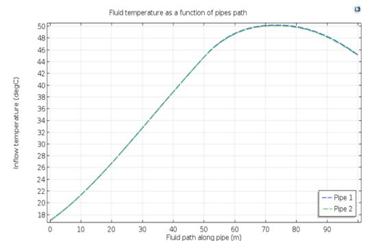
Temperature trend along the pipeline (parallel configuration).
