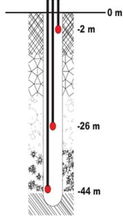
The DHE is a steel pipe, with a total length of 50 meters and a 4,6-mm thickness, considering an outer diameter of 33,7 mm. The flow section has a diameter of 29,1 mm. Pipes location on a cut plane to describe the aquifer dimensions and the temperature trend over depth are available in next figures.
