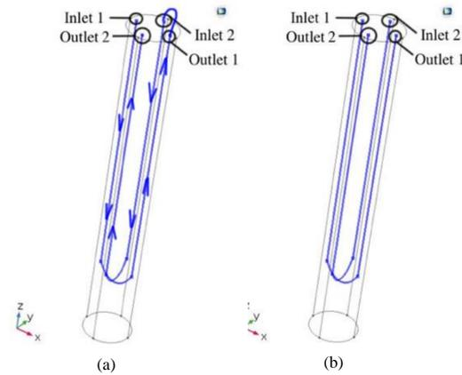
Implemented DHE system geometry configurations of pipes (in blue), not scaled: (a) serial configuration, (b) parallel configuration.
