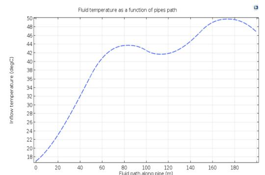
Temperature trend along the pipeline (serial configuration).
